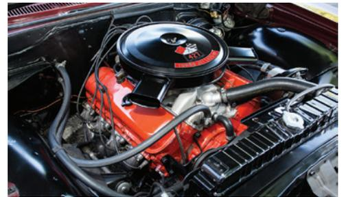
The L72 427 comes with heavy-duty parts like forged pistons and crankshaft, four-bolt mains and rectangle-port cylinder heads. It was only paired to a four-speed manual transmission.
