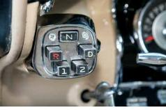
Pushing buttons to shift gears was a radical concept. At night, the button in use was dimmed, while the others around it were brightened.
