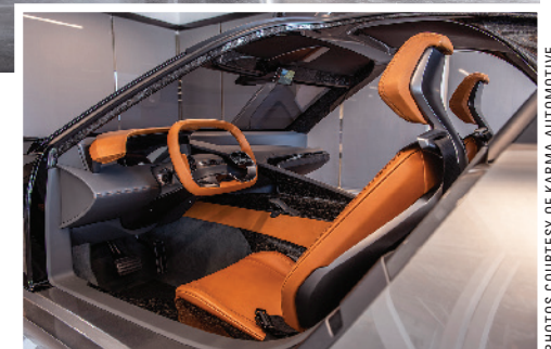
Carbon fiber is used extensively throughout the ultra-clean and modern cabin, which features biometric seats and steering wheel.
